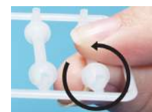
Twisting center post from frame
